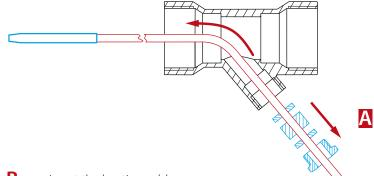
Insert the heating cable. Make the end termination (see QAA-180 (EL-ECMF assembly instructions))
